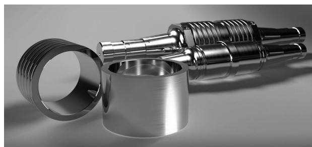
Fig. 2. Roller of small-grade rolling mill for rolling of a reinforcing profile with hard-alloy bandages (a bandage ring in a state of delivery, a bandage ring with the cutted grooves, a steel axis of a roll, the bandaged roll assembled)
