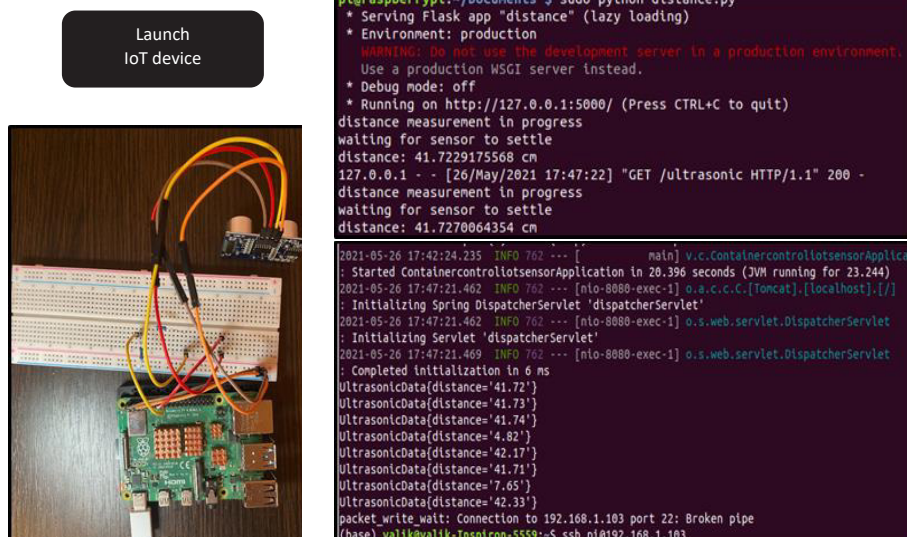
Fig. 4. Prototype of the draft IoT solution for monitoring and analysis of solid waste storage system
