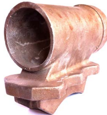
Fig. 2. Casting of high quality in terms of continuity without gating system
