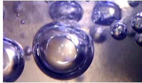
**Fig. 1.** Mirror interfacial surface of bubbles for hydrate-forming gas in water (gas hydrate film is absent)
