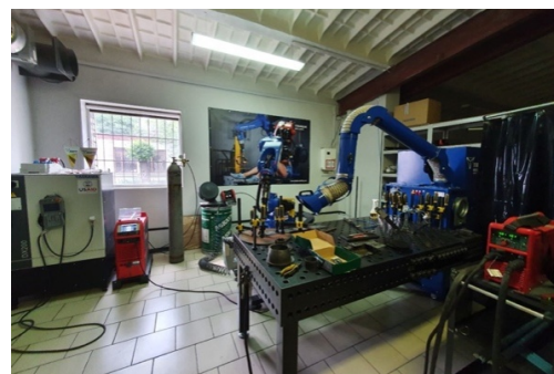
Fig. 1. Robotic WAAM system at Triada LTD Co.
