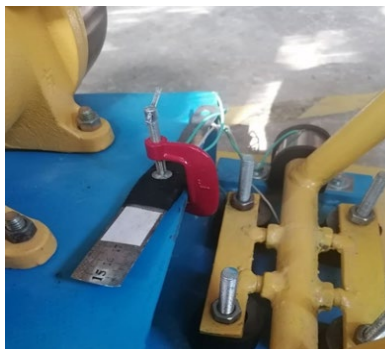
Fig. 5. Fixing the strain gauge on the frame of the vibration plate
