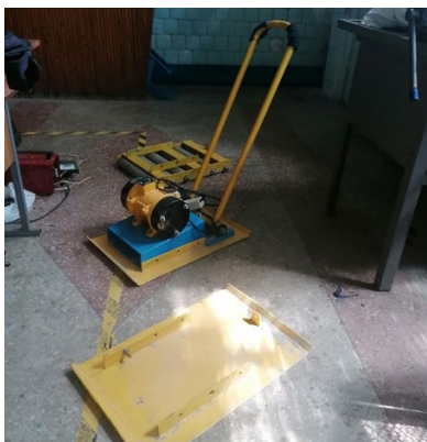
Fig. 6. Vibration plate with replaceable working elements
