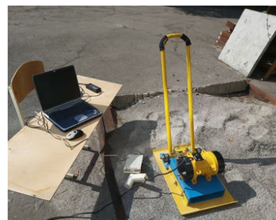
Fig. 8. Measurement of vibration plate effect on the treated medium
