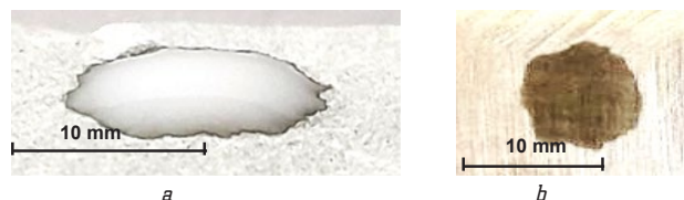
Fig. 4. Photo of the trail of drops: a – aqueous emulsion of gasoline A-95; b – water-organic condensate of tire pyrolysis on the flat surface of clinoptilolite ~3 s after application
