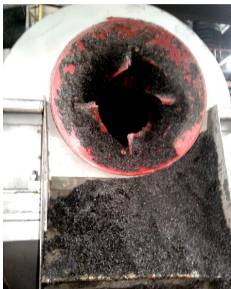
Fig. 3. Classifying tank: a – filter surface of the rotor drum 1.5 mm; b – unloading of filtered sediment by the blades of the screw spirals
