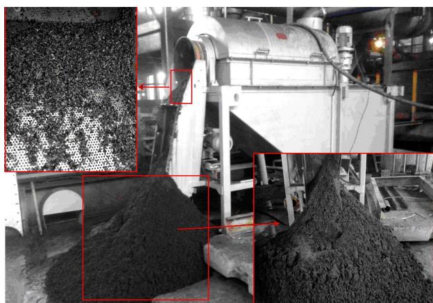
Fig. 4. Unloading of large coal fraction after filtration
