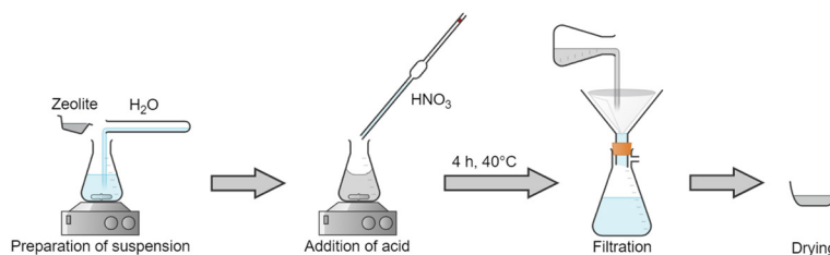
Fig. 1. Schematic representation of the acid activation process of natural zeolite
