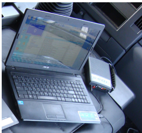
Fig. 1. Application of the G-IDSS device when reading information from the Mymemory unit on the "Ataman" A092N6 bus
