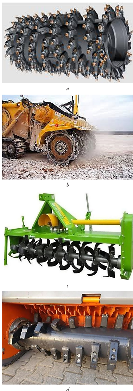
Fig. 1. Rotary working body's: a – road milling machine; b – excavation and milling working body; c – ground cutter; d – forest mulcher
