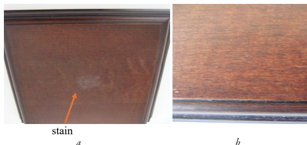
Fig. 5. Samples after water resistance testing:
