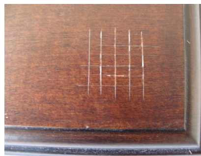
Fig. 1. Sample coated with SU-29 nitro-urethane varnish during adhesion testing
