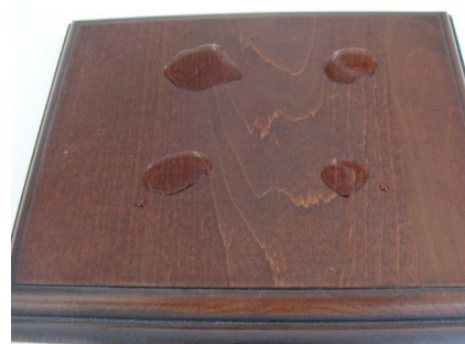
Fig. 3. Testing a sample of varnished wood for staining
