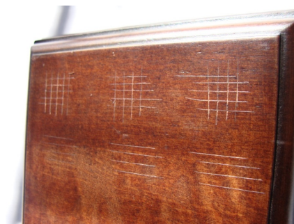
Fig. 2. A wood sample finished with melamine varnish during adhesion testing
