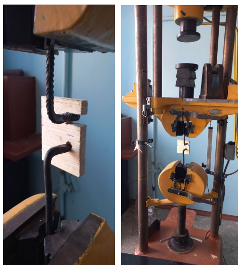
Fig. 3. YMM-20 testing machine with a fixed wood sample
