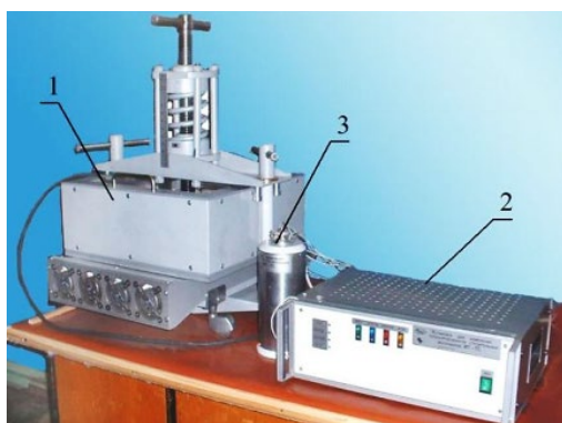
Fig. 6. General view of the laboratory setup for determining the thermophysical properties of alfalfa
