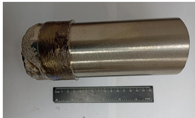
Fig. 4. General view of the secondary \alpha -titanium ingot after removal of the alpha-case layer by turning
