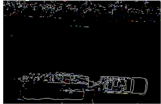
Fig. 7. A segmented test image that is not distorted by speckle noise ( \sigma = 0 ) (Fig. 1), segmented by a method based on the Sobel operator
