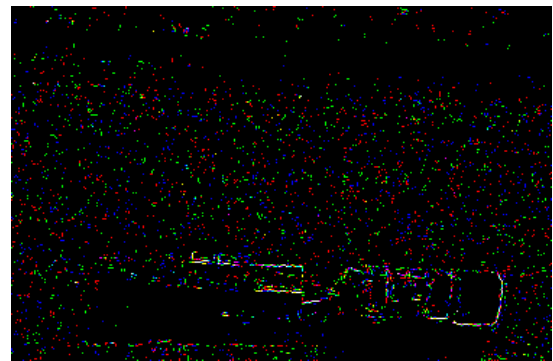
Fig. 8. A segmented test image distorted by speckle noise ( \sigma = 5 ) (Fig. 2), segmented by a method based on the Sobel operator
