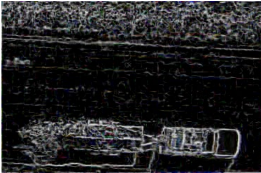
Fig. 4. Segmented test image (Fig. 1) by the method based on the ant algorithm in the absence of speckle noise ( \sigma = 0 )
