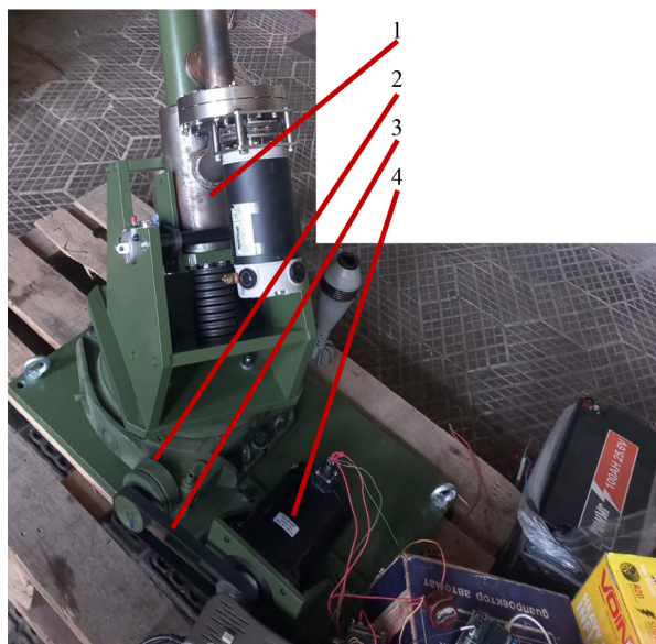
Fig. 1. Drive for turning a gas-detonation mortar: 1 – mortar; 2 – turntable with worm gear; 3 – toothed belt; 4 – stepper motor
