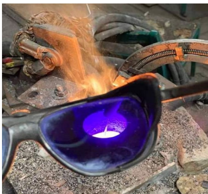
Fig. 2. The process of electroslag surfacing in a CFC at the moment of introducing the wire into the slag bath
