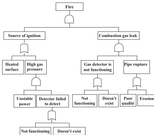
Fig. 13. Application of the fault tree analysis (FTA)
