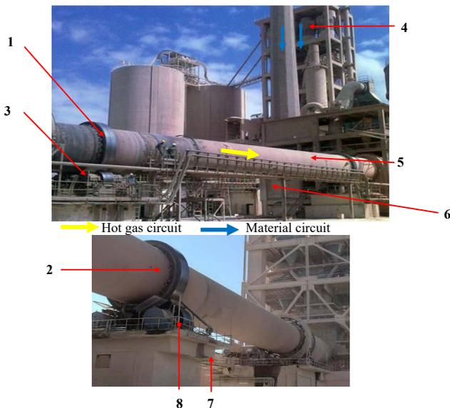
Fig. 1. Components the rotary kiln:
