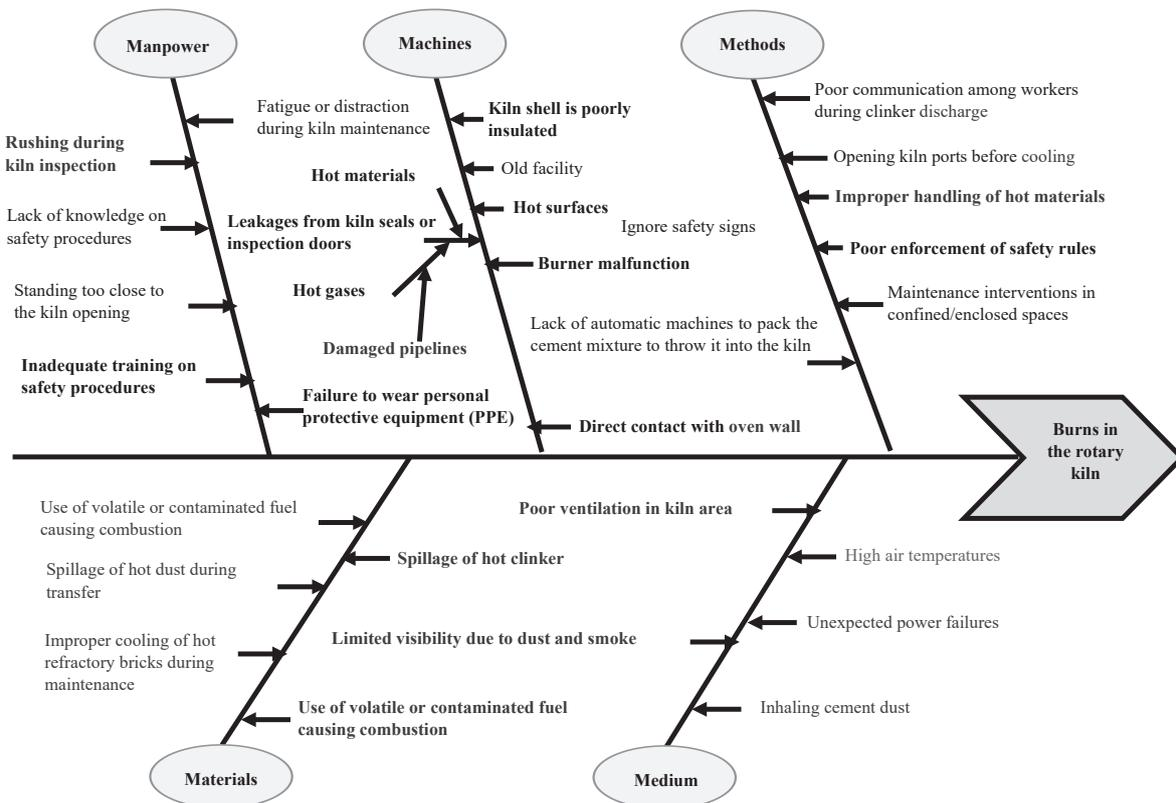
Fig. 10. Possible causes of burns in the rotary kiln to the rule of 5M: Manpower, Machines, Methods, Materials, Medium
