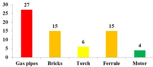
Fig. 11. The criticality levels of the rotary kiln components: 27 – major, 15 – average, 6 – below average and 4 – low
