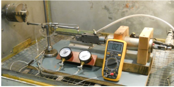
Fig. 7. Laboratory stand for measuring total head and static pressure using a Pitot-Prandtl tube
