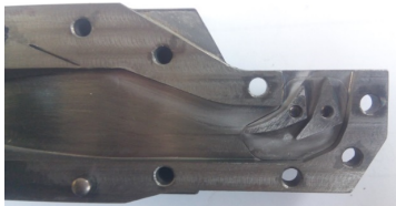
Fig. 9. Trace of particle movement in a gas flow in a 3-channel rotary nozzle
