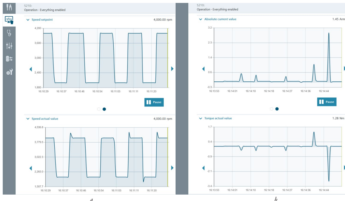
Fig. 21. The process of testing the simulation model using the WEB server "Digital Twin" FC Sinamics S210 (basic values of simulation parameters): a – Speed setpoint and Speed actual value; b – Absolute current value and Torque actual value
