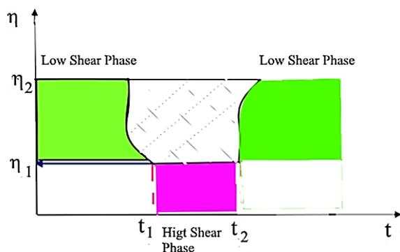
Fig. 1. Dependence of sample viscosity on time with thixotropic behavior:  $\eta$  – viscosity,  $t$  – time
