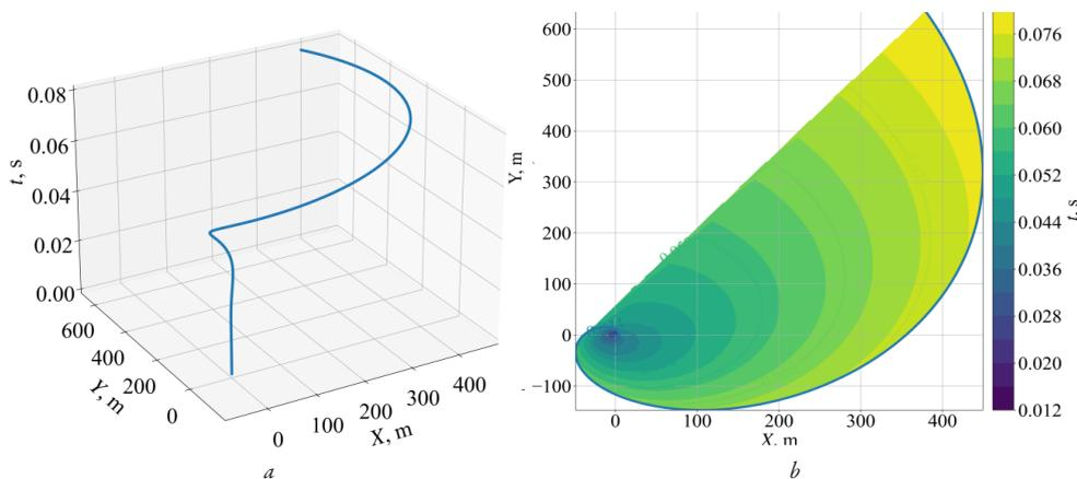
Fig. 2. Parametric trajectory of the granule in the stationary coordinate system: a – three-dimensional space-time representation  $X(t), Y(t)$ ; b – planar trajectory  $X(t), Y(t)$  with time-coded color scale
