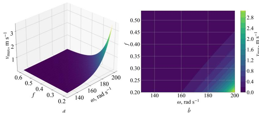
Fig. 3. Maximum velocity of the granule after impact as a function of the rotor angular velocity  $\omega$  and the friction coefficient  $f$ : a – 3D surface representation; b – contour map of  $v_{\max}(\omega, f)$
