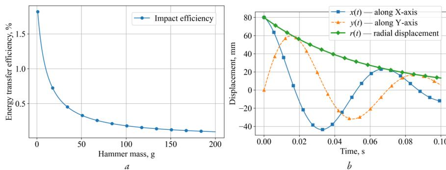
Fig. 4. Energy transfer efficiency and post-impact kinematics of a bee bread granule in the rotating coordinate system: a – dependence of the impact energy transfer efficiency on the hammer mass; b – time evolution of the granule displacement along the  $X$  and  $Y$  axes and the radial coordinate  $r(t)$
