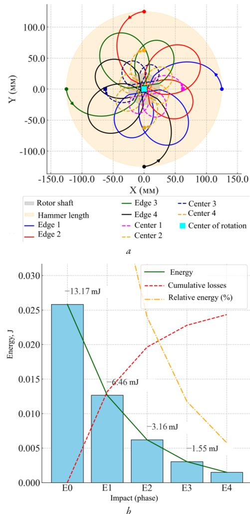
Fig. 5. Post-impact motion and energy dissipation of a bee bread granule during successive collisions inside the rotor: *a* – planar trajectories of the granule projected onto the *OXY* plane for four consecutive impacts; *b* – stepwise decay of the mechanical energy after each impact stage
