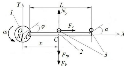
Fig. 1. Schematic diagram of forces acting on the bee bread granule in the contact zone with the hammer (top view): 1 – rotor, 2 – hammer, 3 – granule
