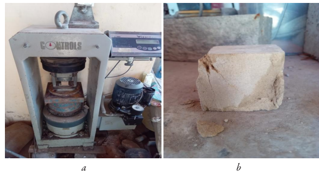
Fig. 4. Specimens crushing tests: a - crushing press; b - specimens after crushing
