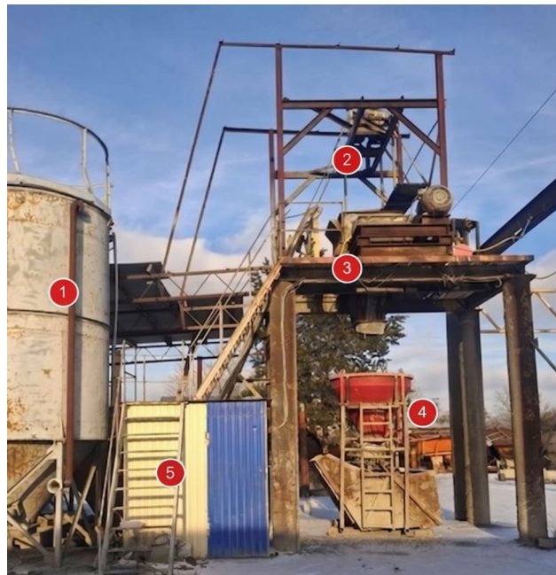
Fig. 1. General view of the "Asfer Group" LLC CMP (60 m 3 /h): 1 – cement silo V = 40 t; 2 – skip lifting mechanism; 3 – forced action mixer; 4 – hopper for receiving and pouring concrete into forms; 5 – control panel
