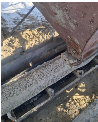
Fig. 2. Adhesion and sticking of wet sand ( W > 5\% ) on the conveyor belt ( W = 6.8\% , CV_Q = 22-25\% )
