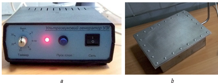
Fig. 2. Ultrasound device photo: a – ultrasonic generator; b – ultrasonic transducer 2 (submersible unit)
