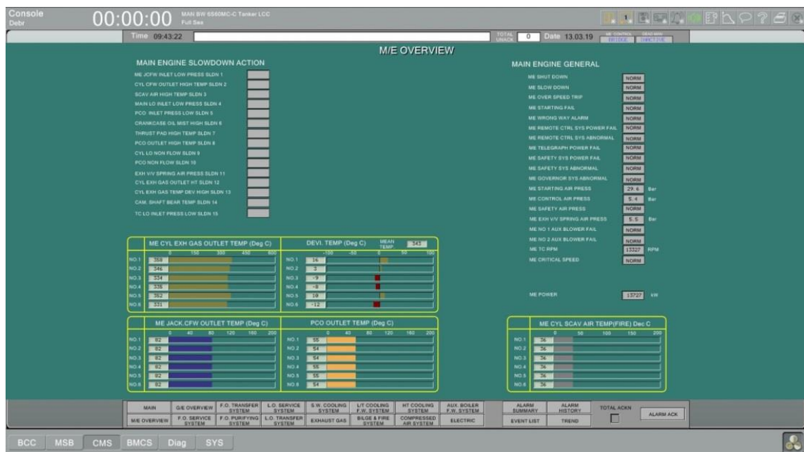
Fig. 5 – Parameters of the main engine without worn piston rings in cylinder #1
