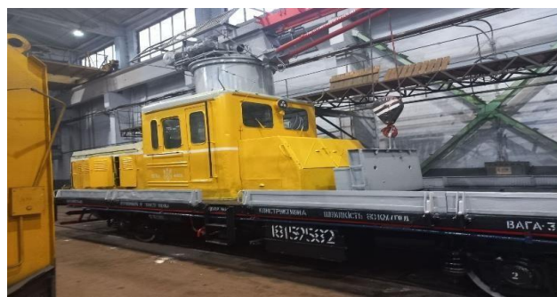
Fig. 2 – Special self-propelled rolling stock type DHK U
