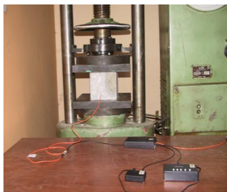
Fig. 3 Laboratory tests of a fiber-optic strain gauge embedded in a concrete cube 150 × 150 mm
